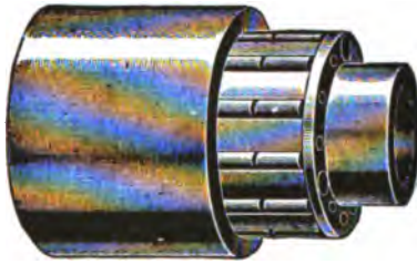
FIG. 468.—Roller Bearings Enclosed in a Retaining Cage. The bearings are hung to the two end pieces of the cage, being separated by stationary pieces of metal. The inner tube is the rotating axle; the outer, the axle box.
